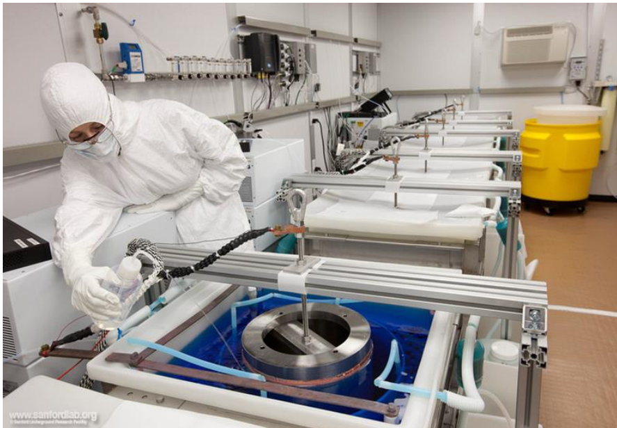
Mandrel insertion in MJD electroforming lab
